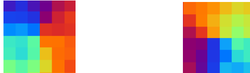
Figure 14: A vortex (left) and an antivortex (right) with colors instead of arrows. As you can see, it is very hard to spot the difference between the two when you only look at the colors.
