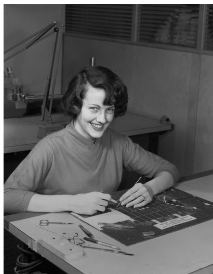
Figure 17: NASA women weaving the core rope ROM and the core RAM for the Apollo mission.
